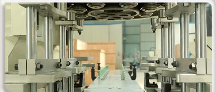
adopt light sectional material and uneasily get deformed can holding jig , combined with servo control, to ensure the fluid and speedy transmission
