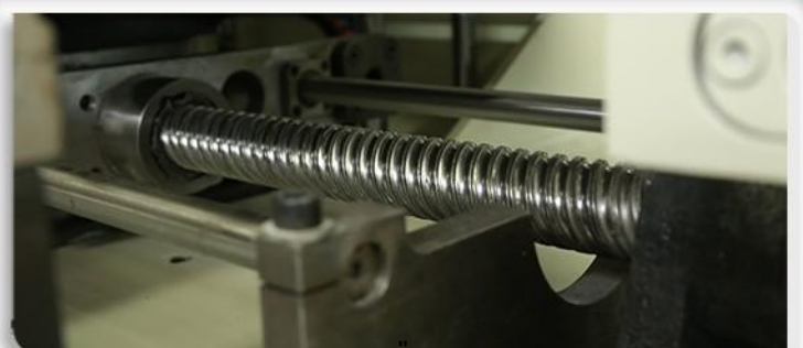
Adopt high-precision imported screw rod and servo motor to ensure the steady and fast conveyance.
