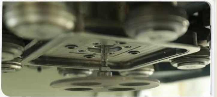
Eight-roller seaming head, can be fastly exchanged between 5-layer and 7-layer.
