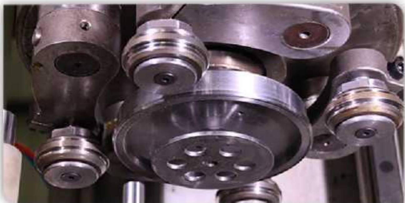
Quick speed seaming head with four rollers
