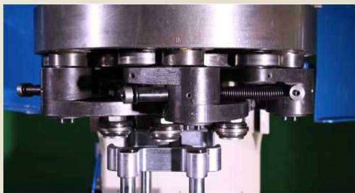
SiX-roller seaming head with steady fast can sealing quality
